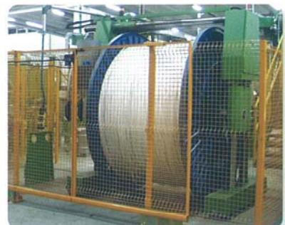
Its right and left movement is driven by an AC motor gear box by means of 4 wheels. The pintles lifting and lowering is driven by two AC motor gear boxes, both synchronised with one push button.
